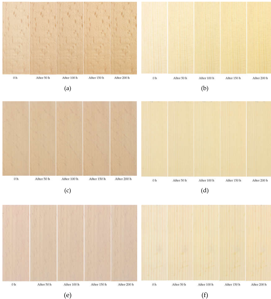
Figure 7. Visual appearance of coated and uncoated samples, before and after 50, 100, 150, and 200 h of UV- irradiation: (a) control beech wood; (b) control pine wood; (c) beech wood coated with polyester/TiO 2 thick film; (d) pine wood coated with polyester/TiO 2 thick film; (e) beech wood coated with polyester/TiO 2 film via (PSP); (f) pine wood coated with polyester/TiO 2 film via (PSP).
