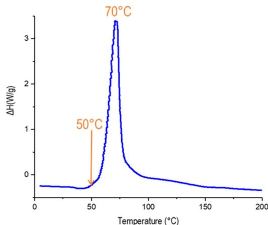
**Figure 7.** DCS evaluation of the thermal initiating ability of Blocbuilder<sup>®</sup> MA (2 wt.%) in Mix-MA; under N<sub>2</sub> (100 mL/min); 10 °C/min; 0–200 °C.
