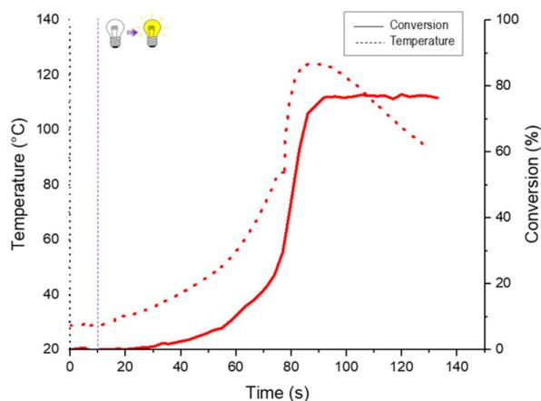
**Figure 8.** Simultaneous RT-FTIR (C=C conversion vs. irradiation time) and thermal imaging (temperature vs. irradiation time) photopolymerization follow-ups (1.4 mm sample) under air upon LED@405 nm irradiation for Mix-MA in the presence of Napht (0.1 wt.%), Ar<sub>2</sub>I<sup>+</sup>PF<sub>6</sub><sup>-</sup> (1.5 wt.%), 4-dppba (0.5 wt.%), and Blocbuilder<sup>®</sup> MA (2 wt.%); irradiation starts after 10 s.
