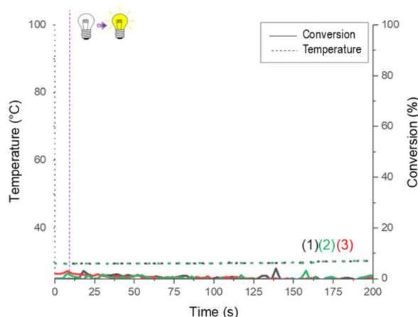
Figure 10. Simultaneous RT-FTIR/thermal imaging photopolymerization kinetics (C=C conversion vs. irradiation time and temperature vs. irradiation time; 1.4 mm sample) under air upon LED@405 nm irradiation for Mix-MA in the presence of (1) monomer alone, (2) Blocbuilder<sup>®</sup>-MA (2 wt.%), and (3) Ar<sub>2</sub>I<sup>+</sup>PF<sub>6</sub><sup>-</sup> (1.5 wt.%), 4-dppba (0.5 wt.%), and Blocbuilder<sup>®</sup>-MA (2 wt.%); the irradiation starts after 10 s.
