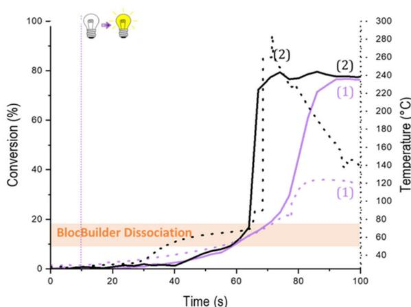
**Figure 13.** Simultaneous RT-FTIR/thermal imaging photopolymerization follow-ups (C=C conversion vs. irradiation time and temperature vs. irradiation time; 1.4 mm sample) under air upon LED@405 nm irradiation in the presence of Napht (0.1 wt.%), Ar<sub>2</sub>I<sup>+</sup>PF<sub>6</sub><sup>-</sup> (1.5 wt.%), 4-dppba (0.5 wt.%), and Blocbuilder<sup>®</sup>-MA (2 wt.%); in (1) Mix-MA; (2) TMPTA; the irradiation starts after 10 s.
