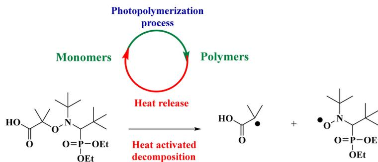
Figure 9. Photopolymerization mechanism.
