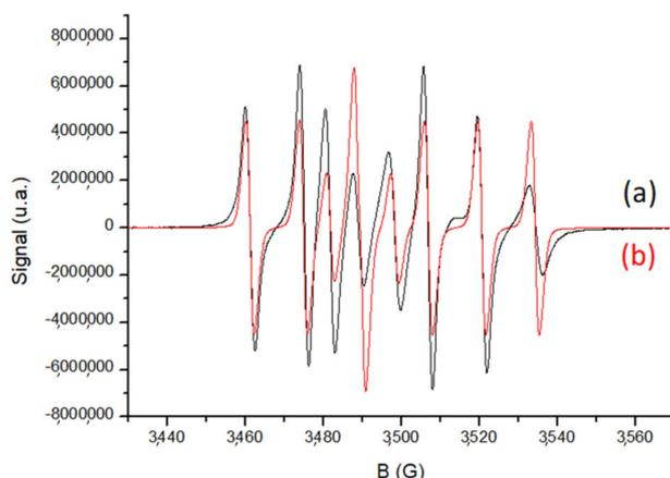
**Figure 11.** ESR-spin trapping spectrum of Napht in combination with Blocbuilder<sup>®</sup>MA Ar<sub>2</sub>I<sup>+</sup>PF<sub>6</sub><sup>-</sup> and 4-dppba in Mix-MA; under air after 15 s of irradiation with an LED@405 nm (110 mW cm<sup>-2</sup>) exposure: (a) Experimental; (b) Simulation of the ESR-spin trapping spectrum of 75% of SG1 radicals ( $a_N = 13.7$  g;  $a_P = 45.7$  g) and 25% of ROO• ( $a_H = 8.2$  G;  $G = 2.011$ ).
