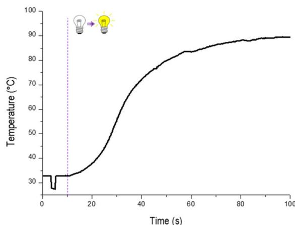
**Figure 6.** Thermal imaging photopolymerization follow-ups (temperature vs. irradiation time; 1.4 mm sample) under air upon LED@405 nm ( $110 \text{ mW cm}^{-2}$ ) irradiation for Mix-MA in the presence of Napht (0.1 wt.%),  $\text{Ar}_2\text{I}^+\text{PF}_6^-$  (1.5 wt.%), and 4-dppba (0.5 wt.%); irradiation starts after 10 s.
