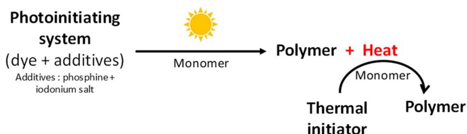
Figure 2. Orthogonal approach between thermal initiation vs. photoinitiation.
