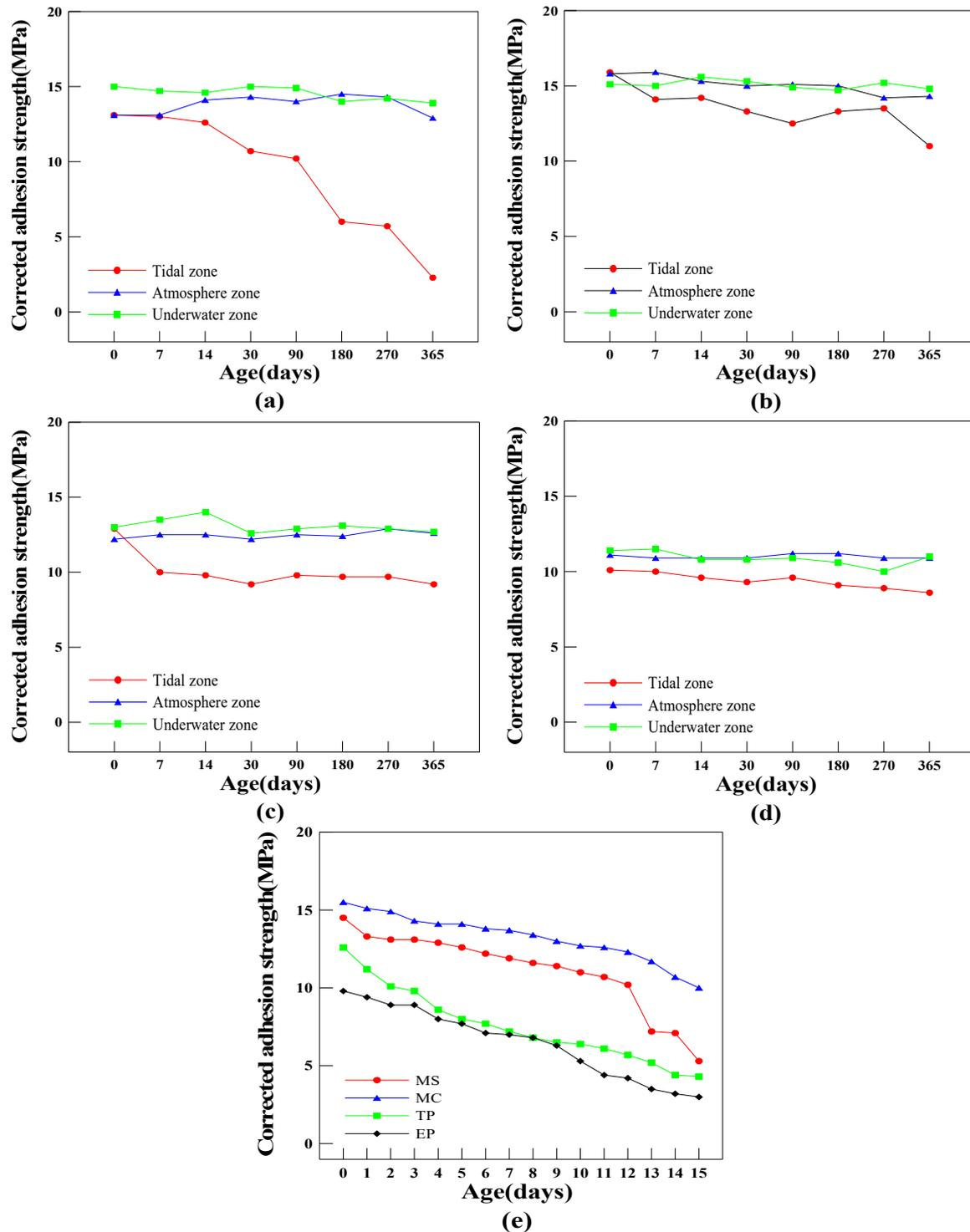
Figure 4. Corrected adhesion strength of (a) MS, (b) MC, (c) TP, (d) EP and corrected adhesion strength of coating systems after salt spray test (e).
