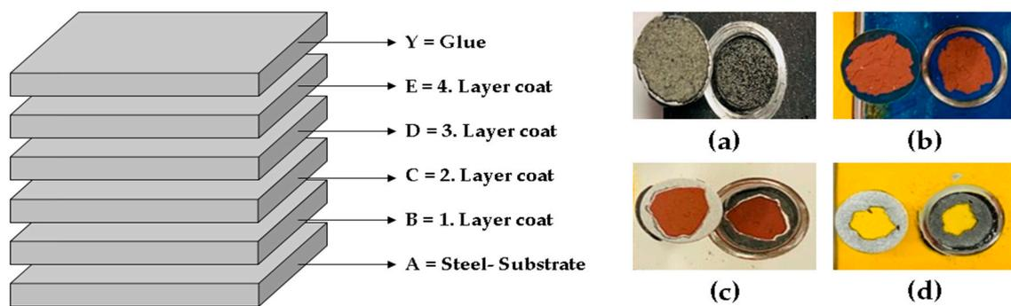
**Figure 3.** Coating layer fracture shape of each coating system: (a) Zn–Al metal spraying (MS), (b) Zn–Al metal spraying + epoxy coat (MC), (c) epoxy coat (TP), (d) epoxy coat + polyurethane coat (EP).
