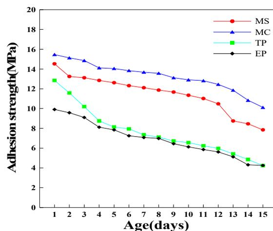
Figure 2. Adhesion strength of coating systems after salt spray test.
