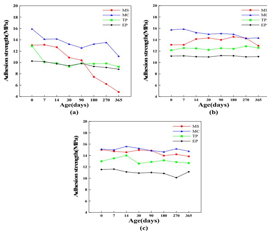
**Figure 1.** Adhesion strength of coating systems exposed to (a) tidal zone, (b) atmosphere zone, (c) underwater zone.
