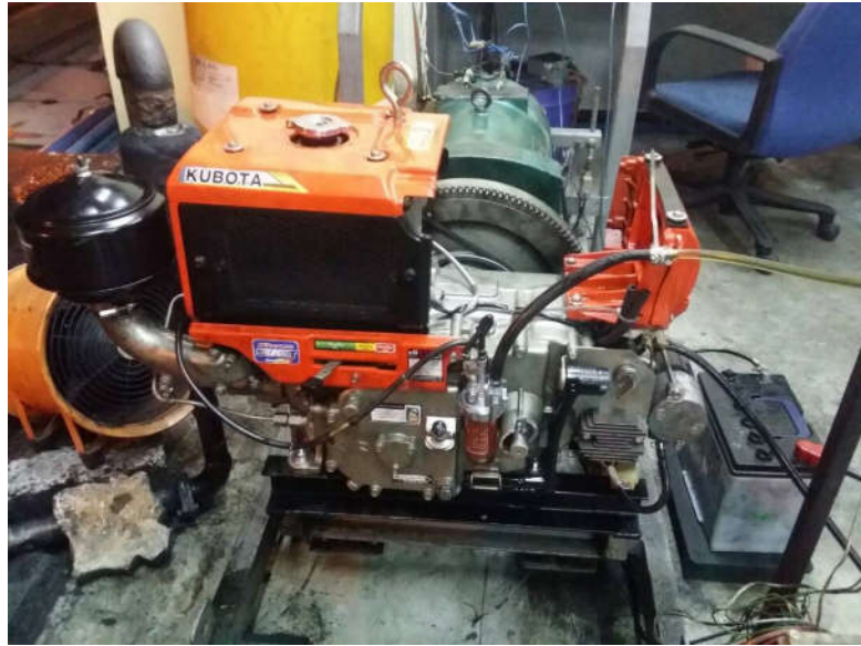
Figure 2. Kubota RT-125 diesel engine experimental setup.
