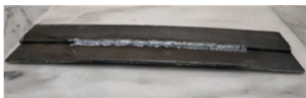
Figure 17. Test sample of optimum weld sequence.
