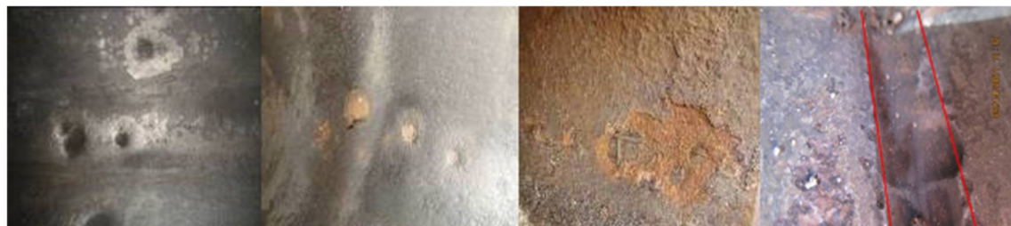
Figure 1. The typical corrosion morphology of the pipes in Tahe Oilfield.
