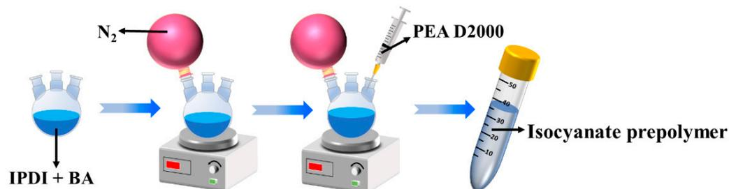
**Figure 1.** Schematic diagram of synthesis of isocyanate prepolymer.
