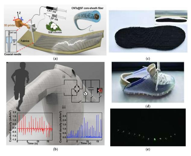
**Figure 3.** (a) Schematic illustration of the 3D-printing process using a coaxial spinneret. (b) Schematic illustration of smart clothes for energy management and their performances [67]. Copyright 2019, Elsevier Inc. (c) 3DP-TENG insole. (d) Photograph of a self-powered lighting shoe with a 3DP-TENG insole inside. (e) LEDs simultaneously lighting while the wearer stomped [68]. Copyright 2019, Wiley-VCH.
