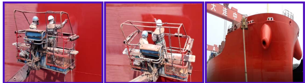
Figure 2. Chinese shipyard painters work at height to paint up-close.
