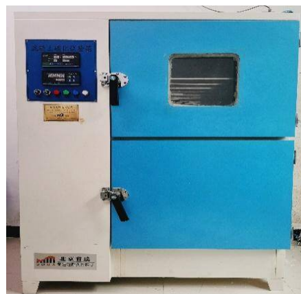
Figure 6. CCB-70F concrete carbonation test chamber.
