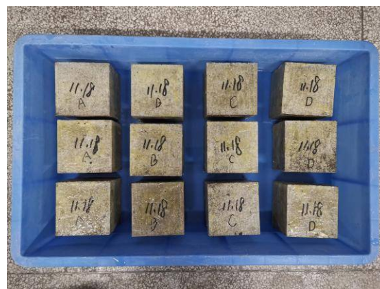
Figure 2. Water absorption test chart (D = not surfaced, A = surfaced with tetraethyl orthosilicate surface treatment agents with acrylic acid, B = surfaced with tetraethyl orthosilicate surface treatment agents with phosphoric acid, C = surfaced with tetraethyl orthosilicate surface treatment agents with hydrochloric acid).
