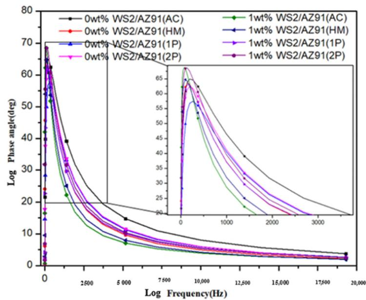
Figure 7. Comparative Bode diagrams for WS<sub>2</sub>/AZ91 composites.
