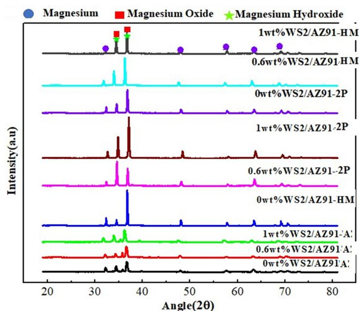
Figure 9. XRD analysis of corroded WS<sub>2</sub>/AZ91 composites.
