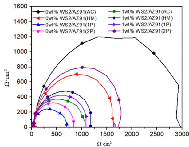
Figure 5. Comparative Nyquist plots for WS<sub>2</sub>/AZ91 composites.
