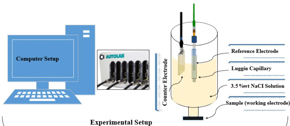
**Figure 1.** Experimental setup for potentiodynamic polarization.
