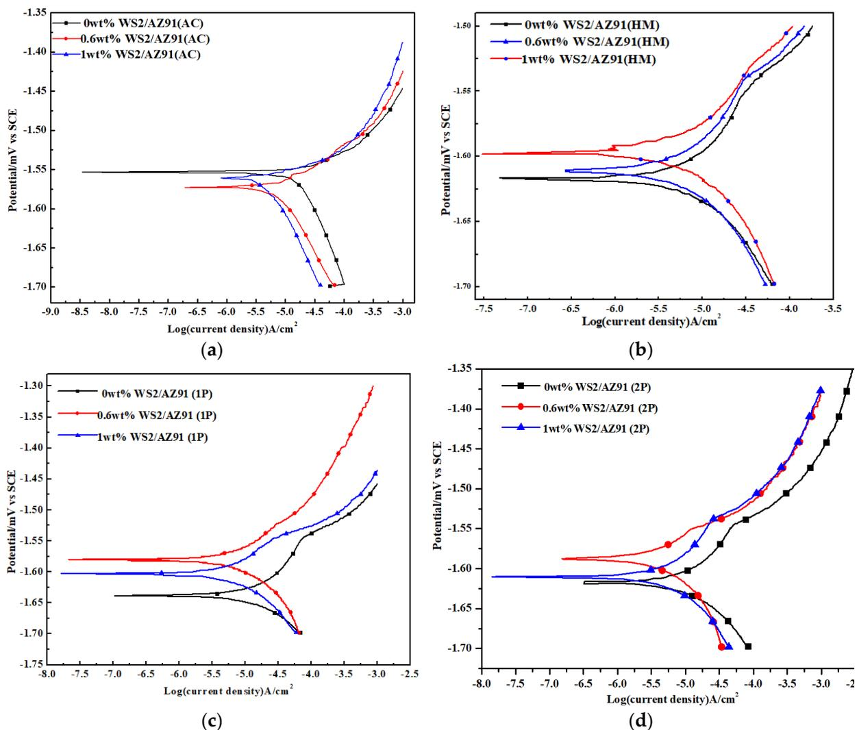
**Figure 2.** Tafel curves for  $WS_2$ /AZ91 composites in (a) as-cast, (b) homogenized, (c) one-pass ECAP, (d) two-pass ECAP.
