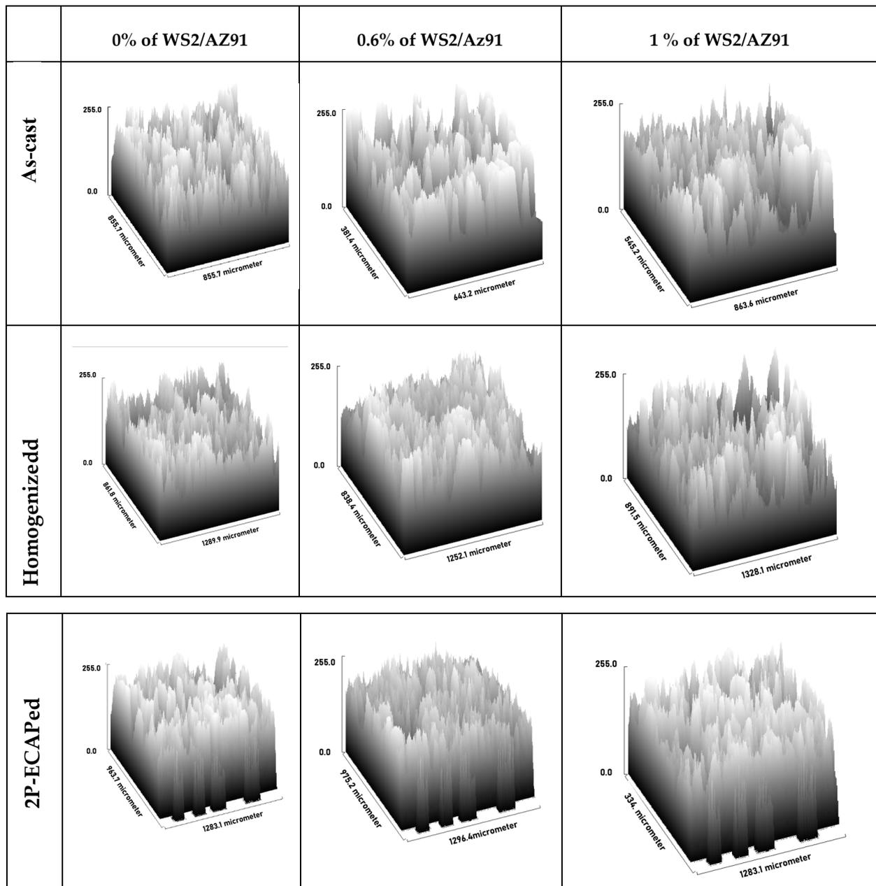
**Figure 8.** Surface roughness generated by SEM images of corroded  $WS_2/AZ91$  samples.
