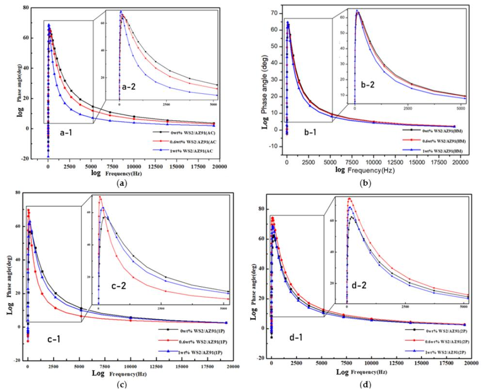
Figure 6. Bode diagrams for WS<sub>2</sub>/AZ91 composites in (a) as-cast, (b) homogenized, (c) one-pass ECAP, (d) two-pass ECAP.
