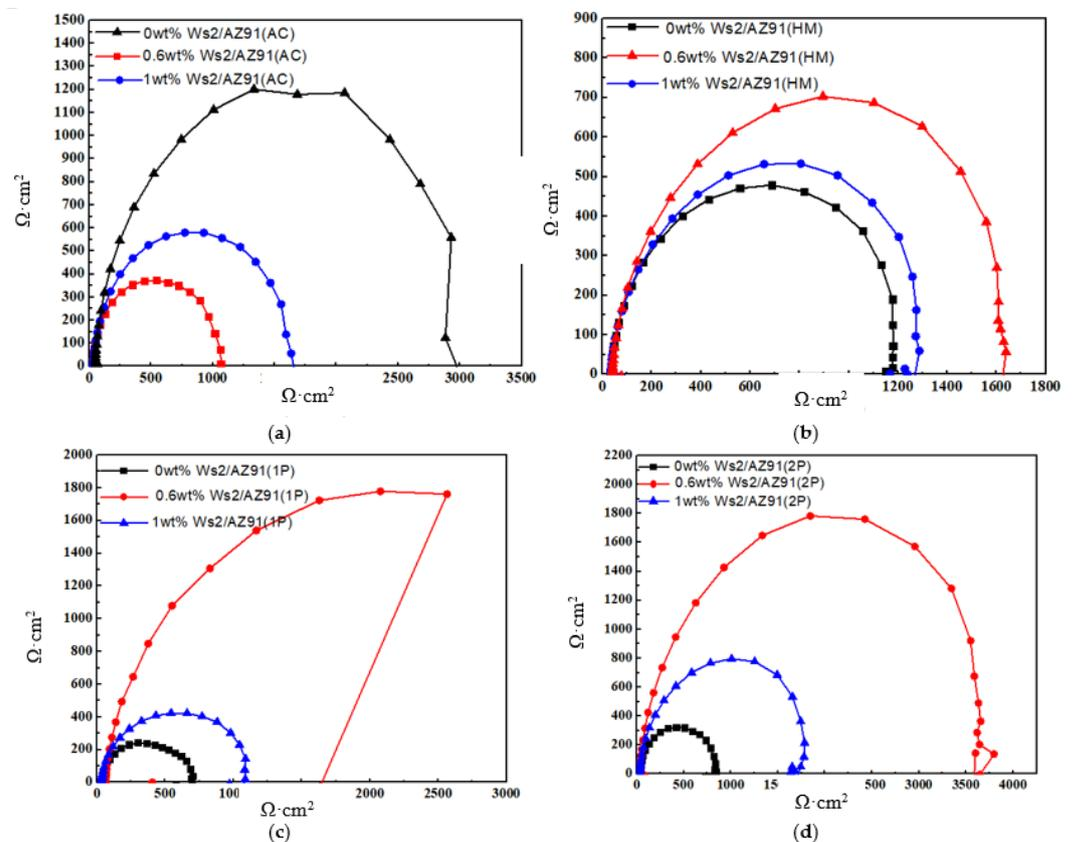
**Figure 4.** Nyquist plots for  $WS_2/AZ91$  composites in (a) as-cast, (b) homogenized, (c) one-pass ECAP, (d) two-pass ECAP.
