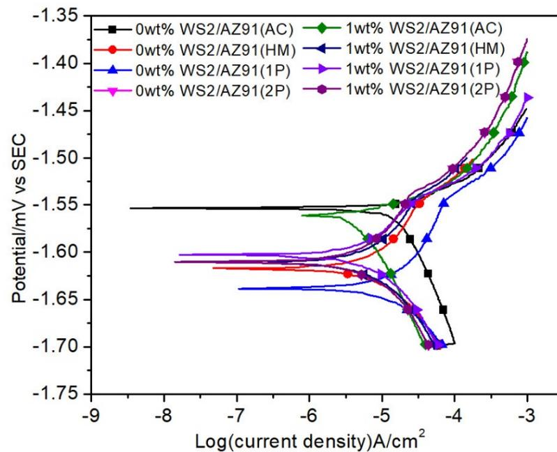
**Figure 3.** Comparative Tafel curves for WS<sub>2</sub>/AZ91 composites.
