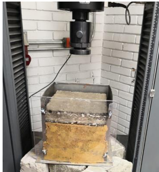
Figure 6. Geometrical configuration of the testing specimen with the granular base as a support.
