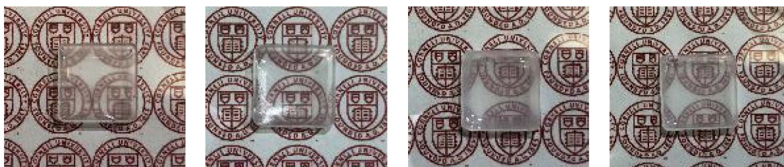
Figure 1. Coatings, 1 cm by 1 cm, cured and removed from PTFE molds. From left to right: control polyurethane, PU-co-1PFPE, PU-co-2PFPE, and PU-co-3PFPE. Coupons were collected from the PTFE mold, and those with bubbles or missing edges were discarded. The samples displayed in this figure reflect characteristics of the larger batch, including size, shape, intact edges, no bubbles present, and visual clarity.
