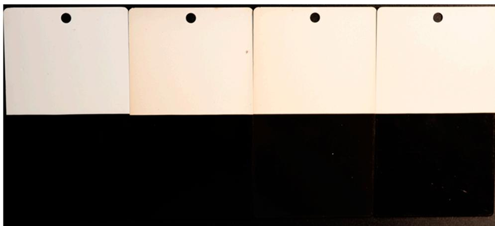
**Figure 7.** The appearance of the coatings containing the four antimicrobial additives, from left to right: Ag-LTA, Ag-Y, Ag-M, and Ag-V.
