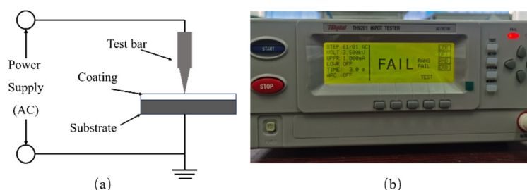
Figure 2. (a) Schematic diagram of breakdown voltage test principle, (b) operation interface of insulation tester.
