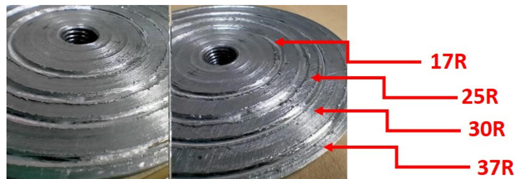
Figure 9. Macro-wear track images developed after wear testing at 17 mm, 25 mm, 30 mm, and 37 mm radii.
