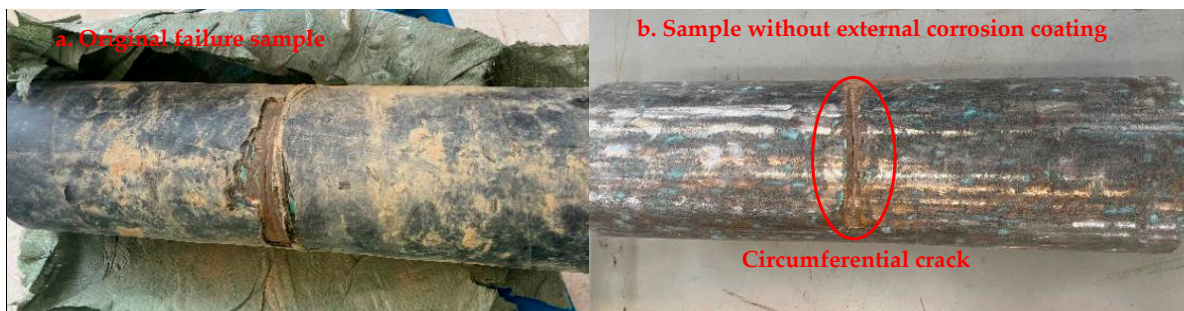
Figure 2. Macroscopic morphology of the outer wall of the failure sample.
