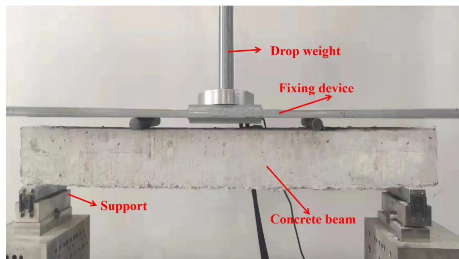
Figure 4. The steel strand-reinforced RPC's impact test.
