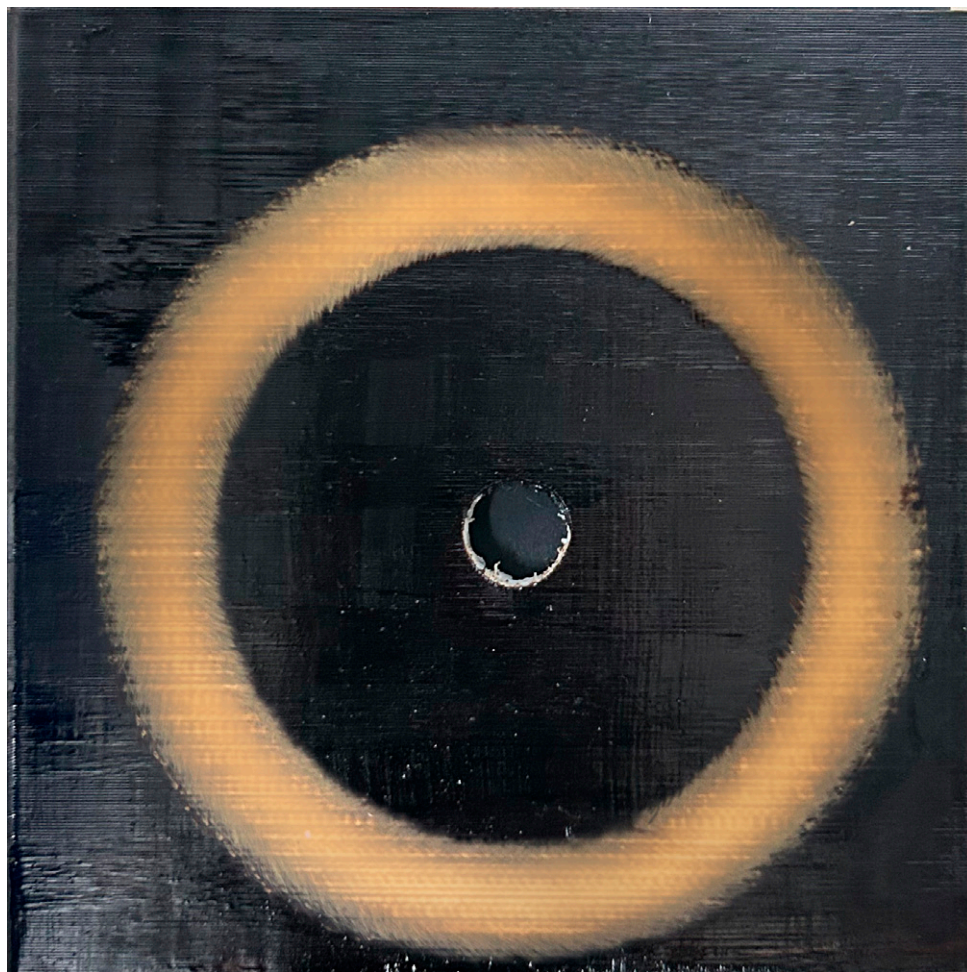
Figure 2. Worn surface morphology of Chinese lacquer-coated PLA specimens after abrasion testing.
