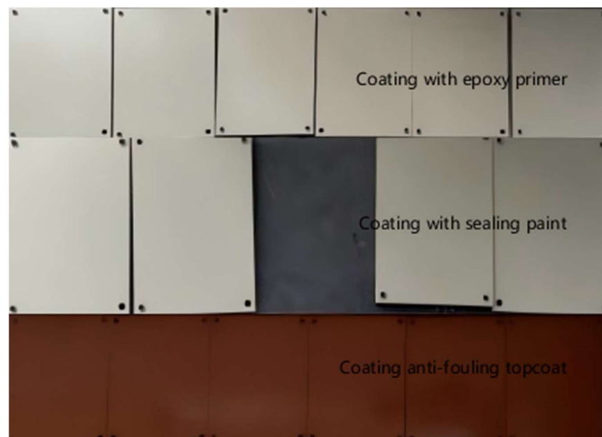
Figure 2. Schematic diagram of the antifouling coating preparation process.
