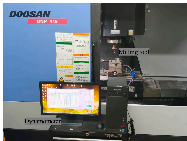
Figure 15. Experimental setup for milling force coefficients measurement.
