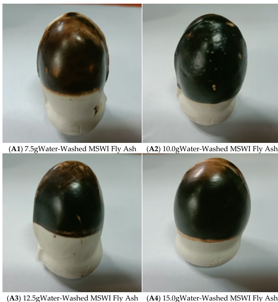
Figure 1. Effect of water-washed MSWI fly ash content on glaze effect.
