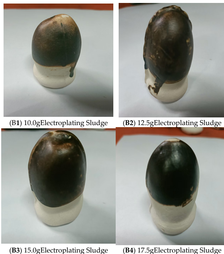
Figure 2. Influence of electroplating sludge dosage on glaze surface effect.
