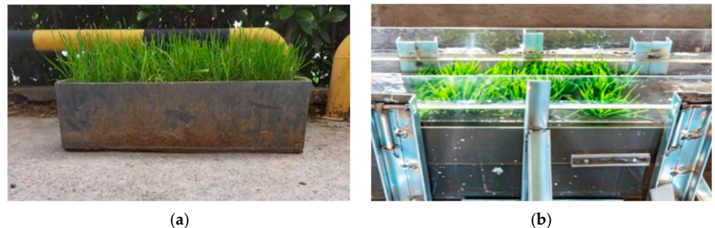
Figure 2. Specimen curing and scouring photographs: (a) specimen curing; (b) specimen scouring.
