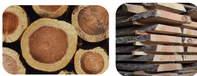
Figure 1. View of the front cut of pine wood before sawing (left); view of the sawn lumber before entering the autoclave (right).
