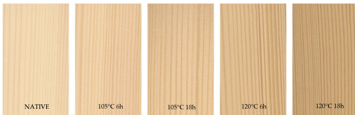
Figure 3. The color of pine wood in the steaming process.
