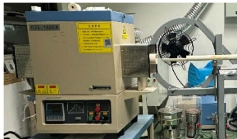
Figure 1. GSL 1600X resistive tube furnace.
