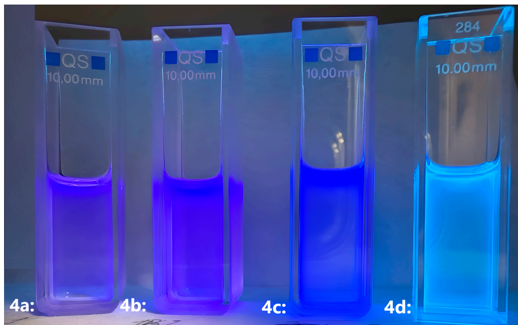
Figure 1. Observed luminescence of 2,6-bis(oxazolo[5,4-b]pyridin-2-yl)pyridine samples under UV irradiation.
