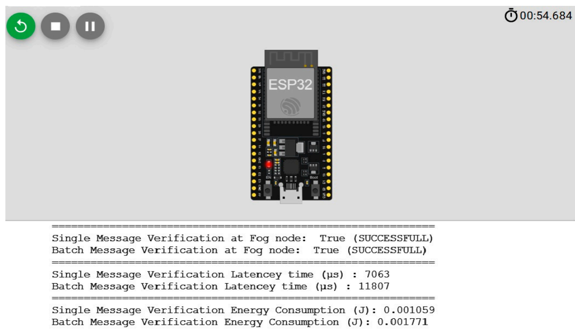
Figure 12. Simulation result showing latency time and energy consumption for single message verification and batch verification.
