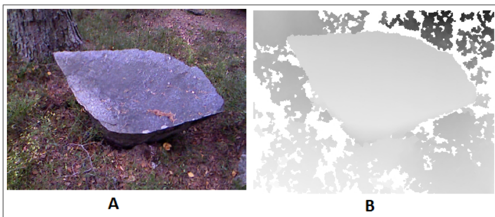
Figure 6. RGB (A) and depth (B) image of stone using Microsoft Kinect.
