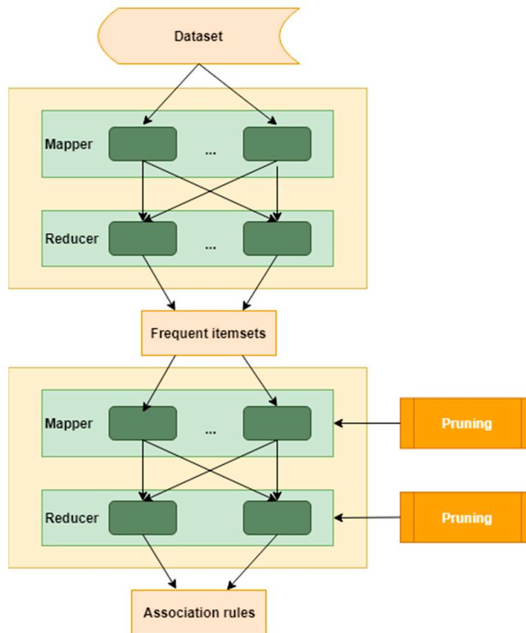
**Figure 1.** Flow diagram of the improved Apriori algorithm.
