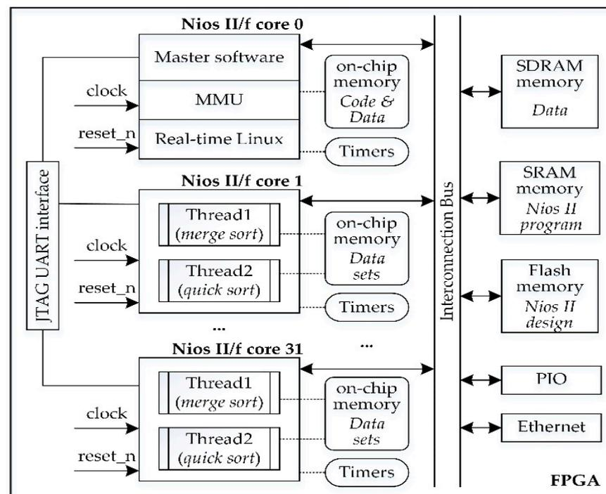
**Figure 1.** The 32-core system architecture.
