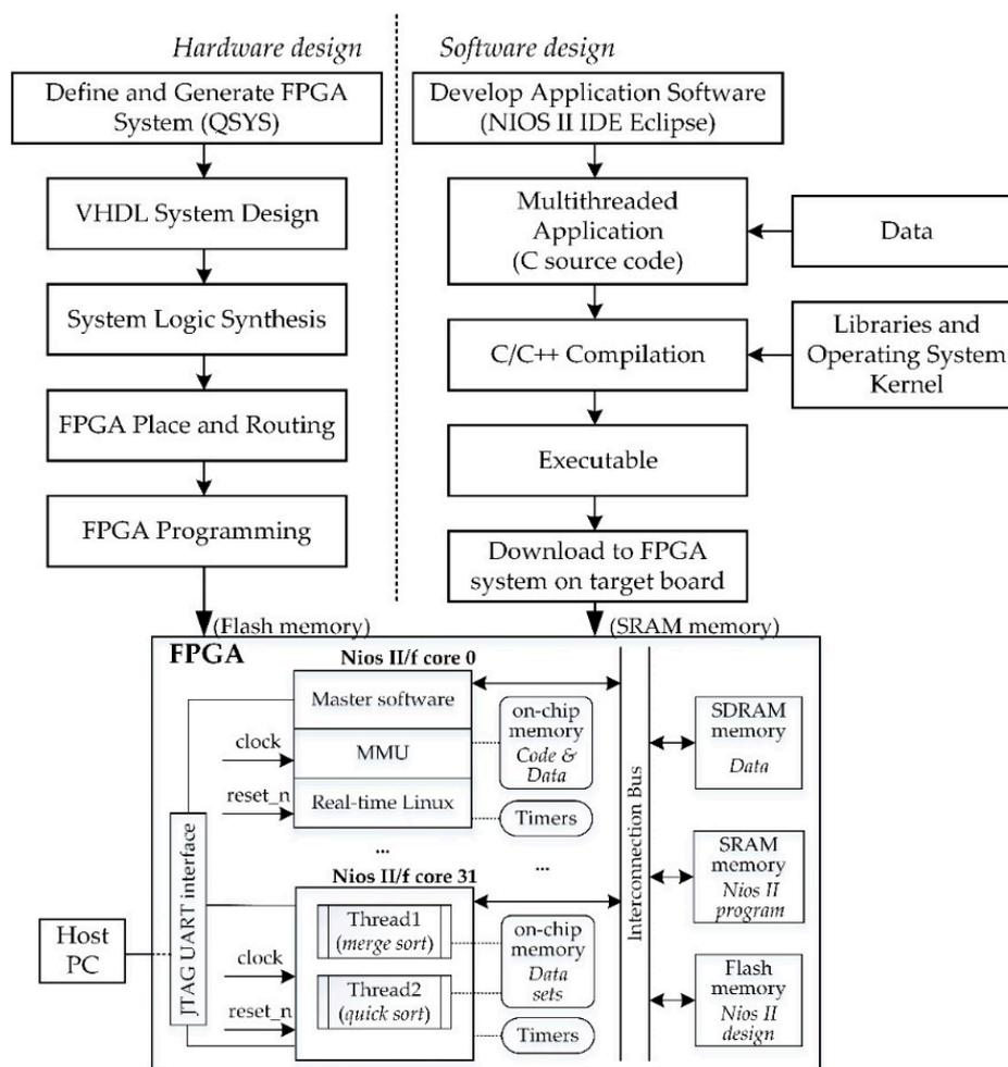
Figure 2. Hardware and software co-design flow and system infrastructure.
