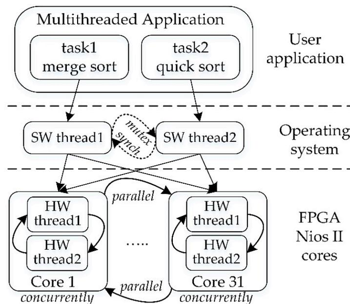
**Figure 4.** Execution flow of the multithreaded application.
