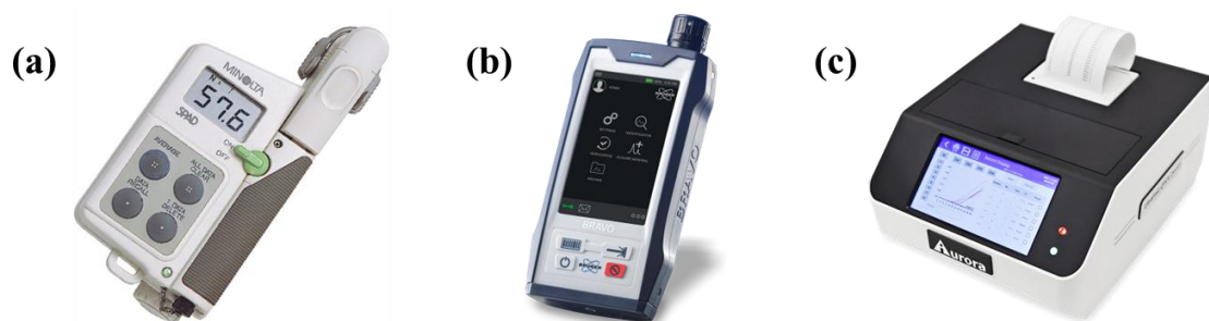
Figure 7. Examples of handheld tools used for crop health monitoring: (a) SPAD 502 chlorophyll meter [102]; (b) BRAVO handheld Raman spectrometer [103]; (c) compact qPCR device (Aurora) [104].
