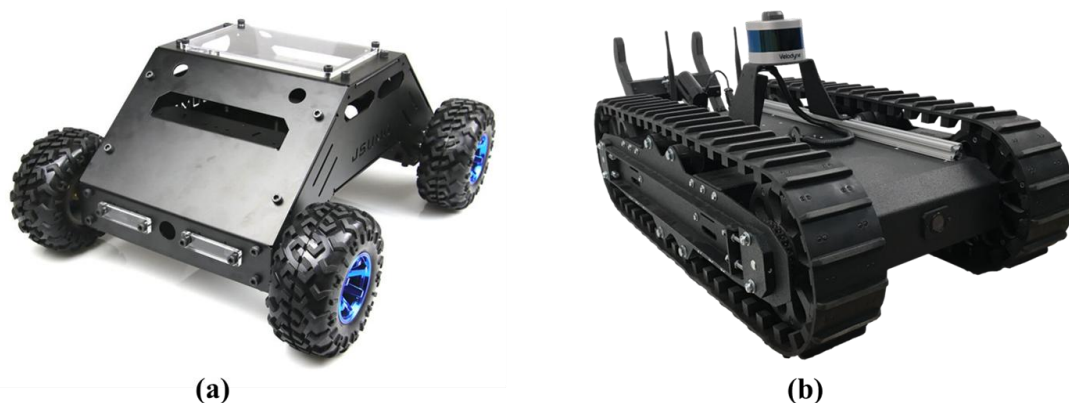
Figure 9. Two major wheel configurations of UGVs used in agriculture: (a) wheel-type UGV (Atlas 4 × 4 All Terrain Explorer Robot) [136]; (b) track/crawler-type UGV (SuperDroid HD2 Treaded ATR) [137].
