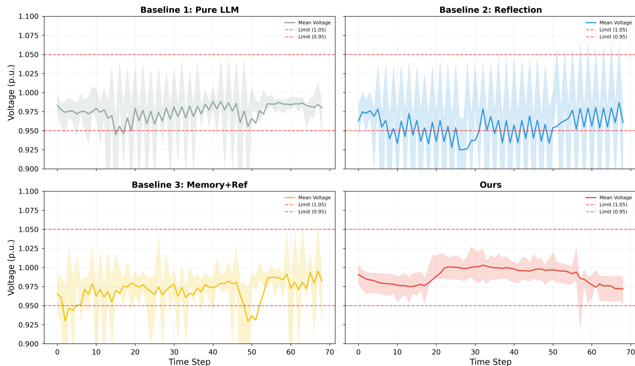
Figure 4. Voltage safety profile comparison over time. The solid line represents mean voltage, and the shaded area indicates voltage standard deviation.
