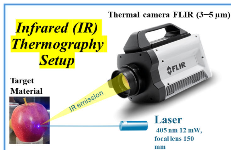
Figure 1. Schematic representation of the IR thermography setup.
