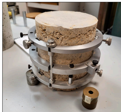
Figure 9. CBGM CBR sample using ring extensometer.
