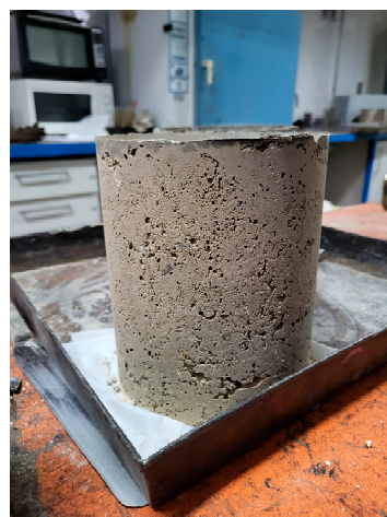
Figure 1. CBR sample of CBGM containing 3% ACS and 2% PC.
