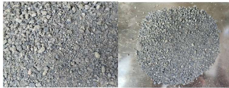
Figure 2. Physical appearance of the recycled fine aggregate (RF, 0–5 mm) used in this study.
