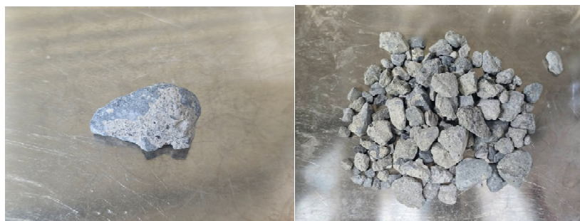
Figure 1. Physical appearance of the recycled coarse aggregate (RC, 5–20 mm) used in this study.
