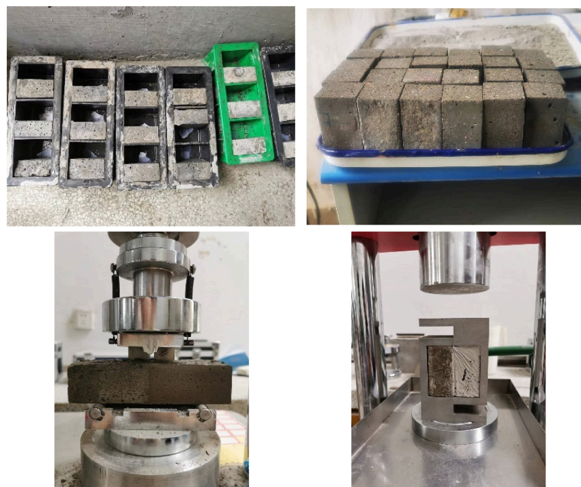
Figure 3. New and old mortar bonding specimens and field test equipment.
