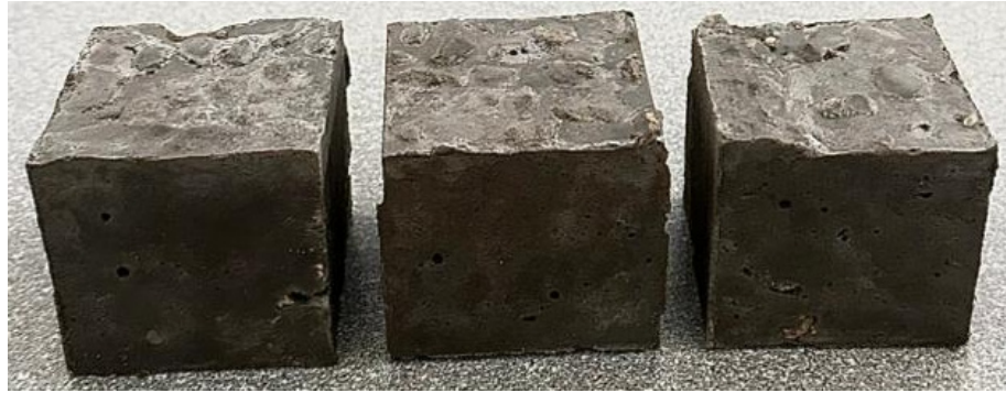
Figure 5. Lightweight cementitious composite specimens containing sintered fly ash aggregate after 7 days of curing.
