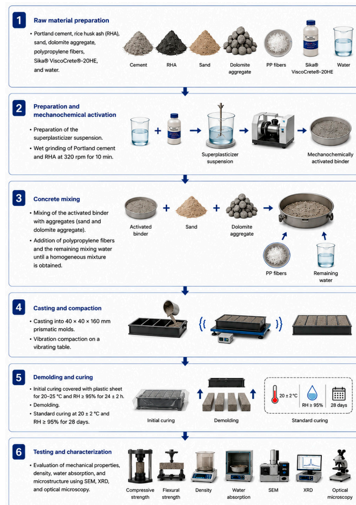
Figure 3. Simplified process flow for the preparation, curing, and characterization of concrete incorporating a mechanochemically activated rice husk ash-based organomineral modifier.
