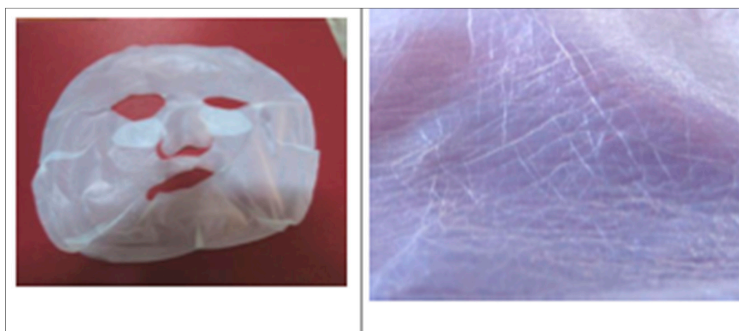
Figure 2. left: unfolded face placebo mask (PM); right: pattern of microfibrils network.
