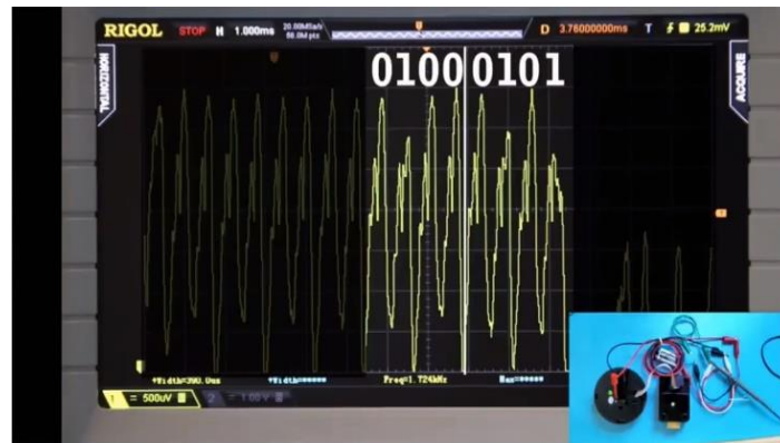
Figure 5. SPA readout of lock keycode [28].
