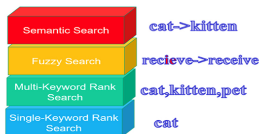
Figure 1. The hierarchy of standard searching modes and the concrete associated examples. Unlike single and multi-keyword rank search, fuzzy and semantic search belong to high-level searching modes.
