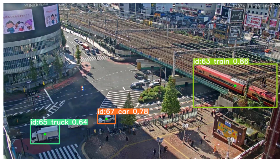
Figure 5. The perception layer of Pipeline C running on a public urban traffic-camera feed. A YOLO-family detector returns persistent identifiers and class labels for vehicles in the frame (here, a car, a truck, and a train). Cross-frame trajectory data from these detections is the input to the pipeline's Extract stage in Figure 4. Source: frame captured by the authors from a publicly accessible traffic-camera broadcast feed; reproduced for academic-illustrative purposes.
