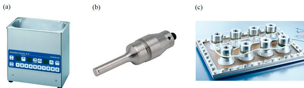
Figure 13. Different types of ultrasound generators: (a) ultrasonic bath [77], (b) ultrasonic horn [78], and (c) ultrasonic plate transducer [79].
