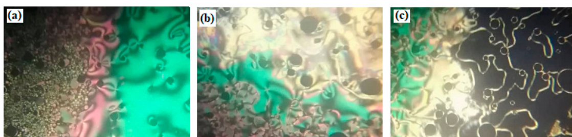
Figure 3. Nematic phase textures during heating under polarized optical microscopy (POM) of 1:2 HBSMC, A/2B12 (a) at 83.0 °C, (b) at 91.0 °C, and (c) at 95.0 °C.
