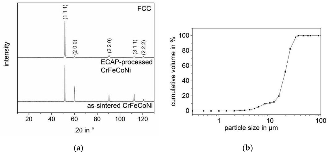
**Figure 2.** Results of diffractometry; (a) X-ray diffraction (XRD) diffractogram of the as-sintered and ECAP-processed materials, (b) cumulative particle size distribution of the atomized CrFeCoNi powder.
