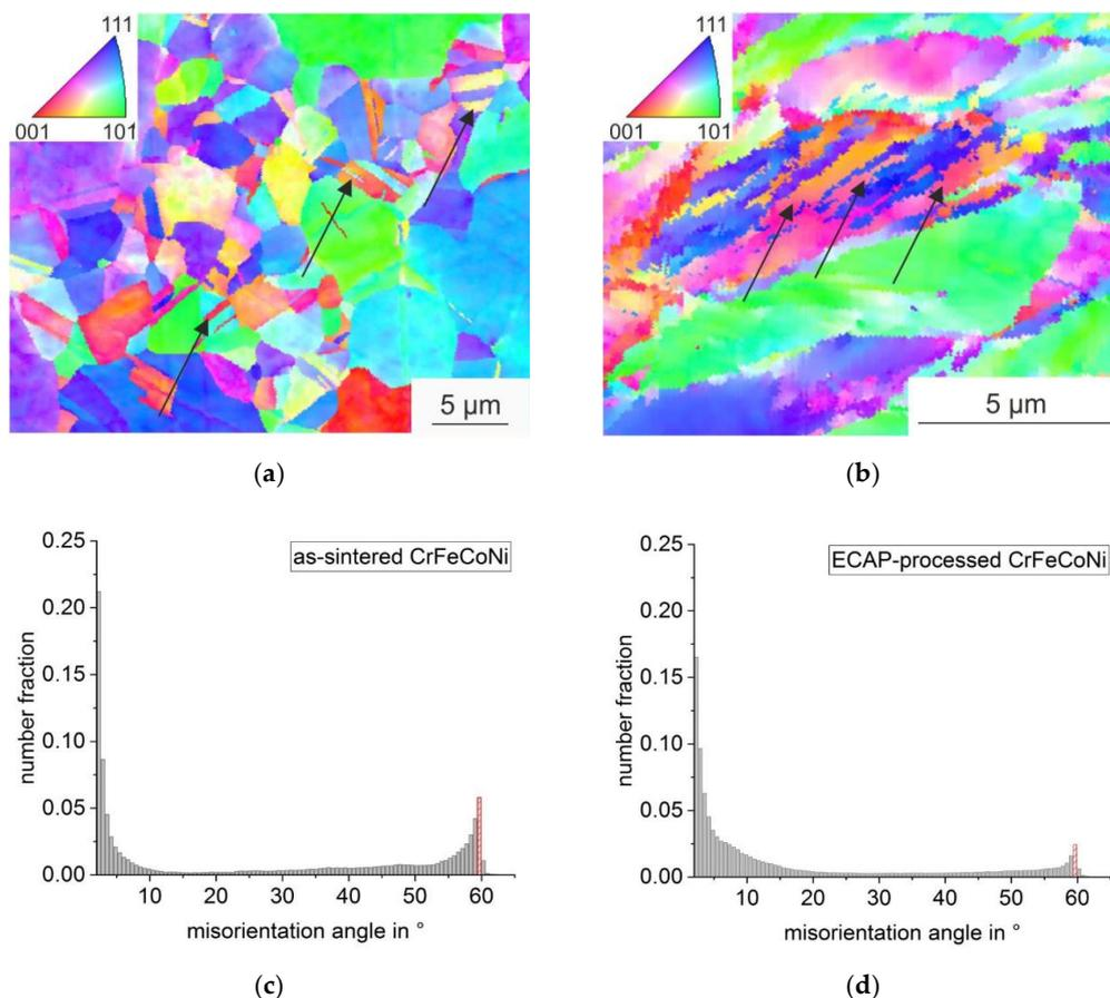
**Figure 5.** Results of EBSD measurements; orientation maps (OM) of the (a) as-sintered and (b) ECAP-processed CrFeCoNi as well as (c,d) the misorientation angle distribution. Twins are marked with black arrows in (a,b).
