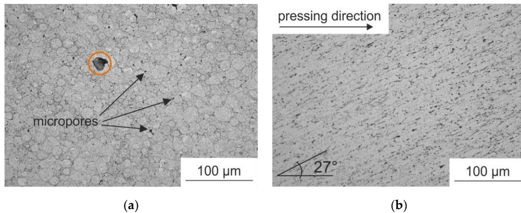
**Figure 3.** Optical microscopy images of etched (a) as-sintered and (b) ECAP-processed CrFeCoNi. In (a), some micropores are exemplary visible (marked with arrows). In the orange circle (a), a broken particle resulting from the metallographic preparation can be seen. After ECAP-processing, the former powder particles are elongated.
