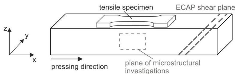
**Figure 1.** Schematic illustration of the equal-channel angular pressing (ECAP) billet. The pressing direction (parallel to the length axis of the die's exit channel), the plane of the microstructural investigations and the ECAP shear plane within the ECAP billet are marked.
