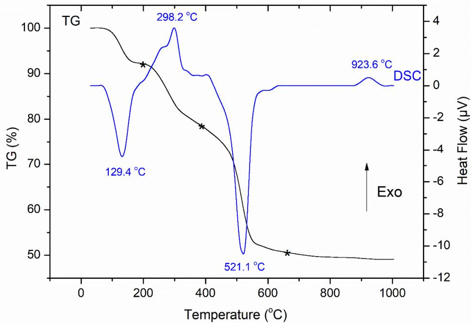
**Figure 1.** Thermogravimetry–Differential Scanning Calorimetry (TG–DSC) curves of the as-sintering bioactive glass sample.
