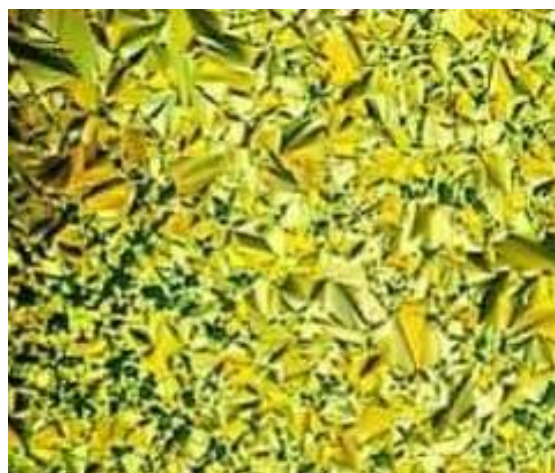
Figure 2. POM smectic A texture of the derivative III during heating scan at 50 °C.
