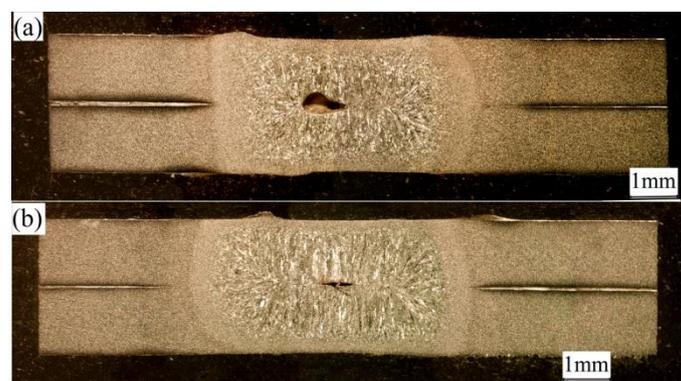
**Figure 9.** The geometric properties of the welded joints in the electrode failure process: (a) the 528th weld; (b) the 616th weld.
