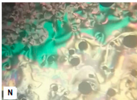
Figure 2. Nematic texture of I_8 derivative upon cooling round at 99^\circ\text{C} under POM.
