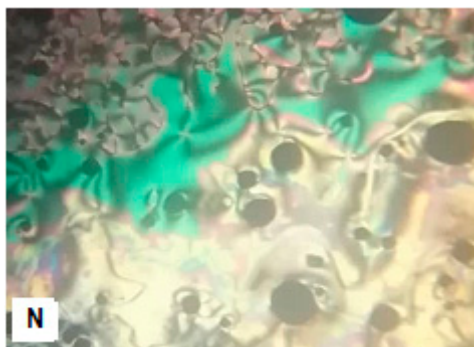
Figure 2. Nematic texture of I_8 derivative upon cooling round at 99 °C under POM.
